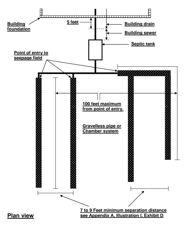
Section 905.ILLUSTRATION J Septic Tank Subsurface Seepage Field
