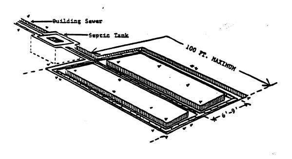
Section 905.ILLUSTRATION J Septic Tank Subsurface Seepage Field
