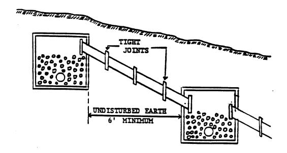
\*\* Differing ground slopes over subsurface disposal fields may require use of various combinations of fittings.
