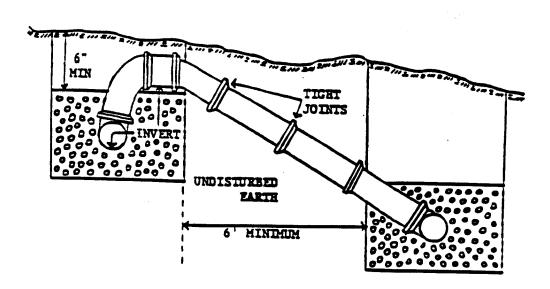
NOTE: Invert of the first relief line must be at least 1 inch lower than invert of the septic tank outlets.
