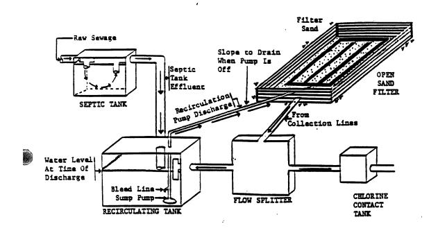
Section 905.ILLUSTRATION O Re-circulating Sand Filter System
