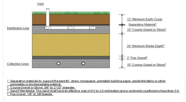
Section 905.ILLUSTRATION O Re-circulating Sand Filter System
