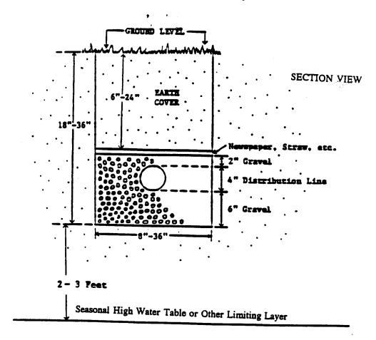
Section 905.ILLUSTRATION J Septic Tank Subsurface Seepage Field
