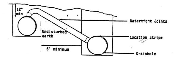
NOTE: Invert of the septic tank outlet shall be at least one inch higher than the top of the gravelless pipe.
